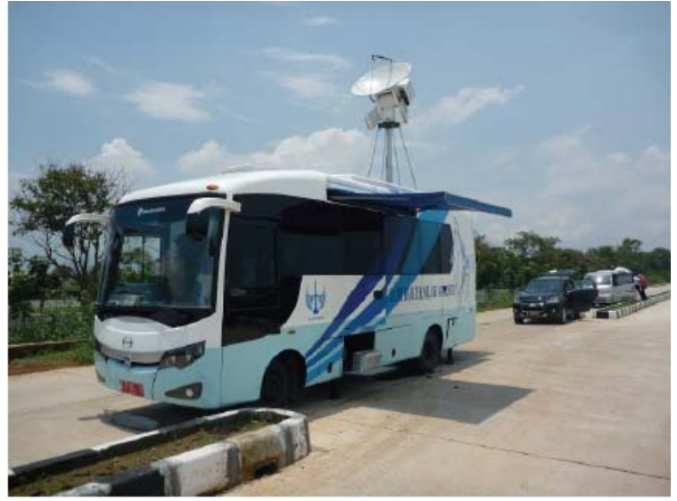
(2) GMWR – 25 radar installed on the LAPAN research bus
